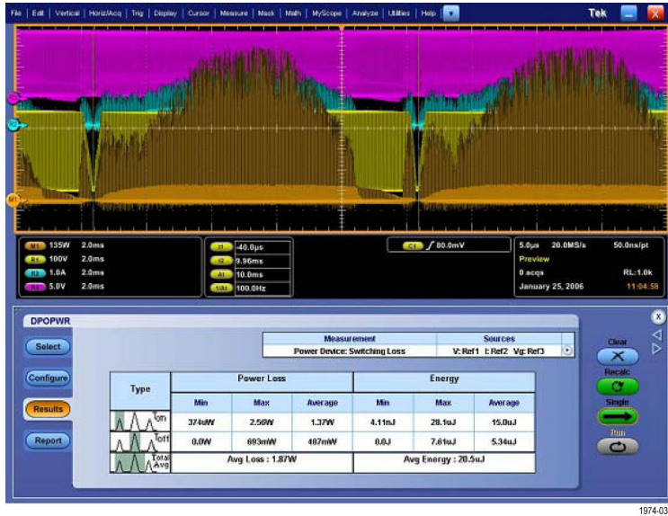
Figure 3: Switching loss results display
